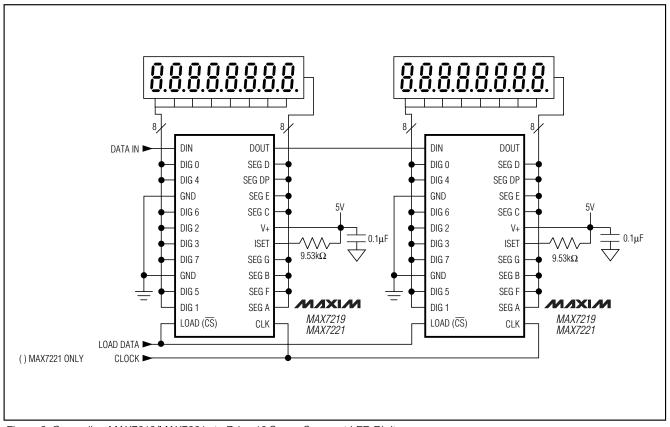
Figure 3. Cascading MAX7219/MAX7221s to Drive 16 Seven-Segment LED Digits
