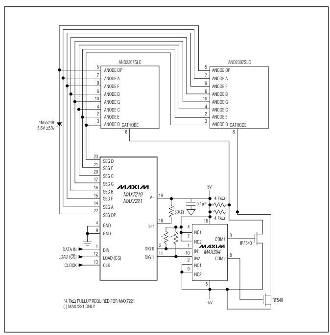
Figure 2. MAX7219/MAX7221 Driving 2.3in Displays
